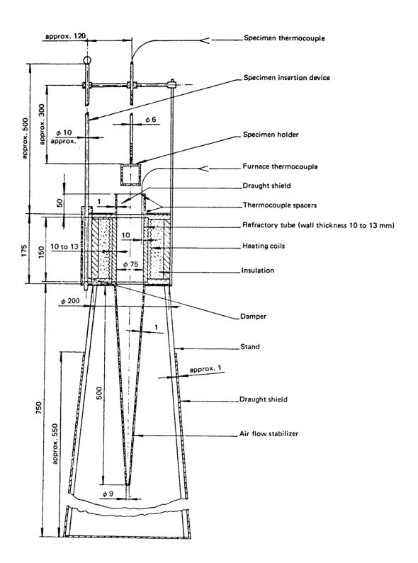
FIGURE 1 - General arrangement: Non-combustibility apparatus
